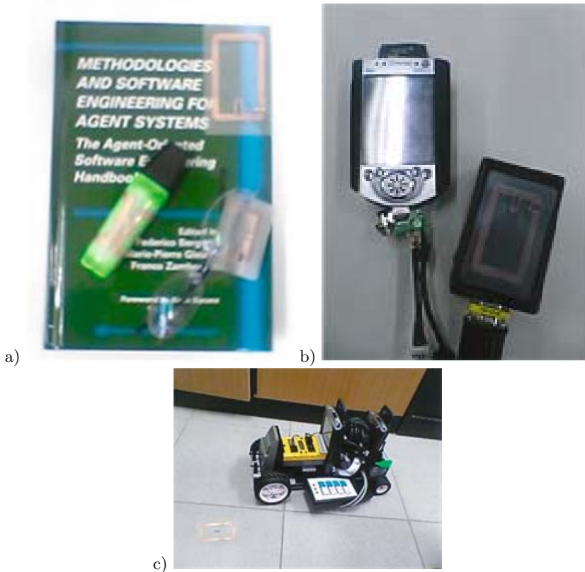
Fig. 3. (a) Our test-bed hardware implementation. (b) Some tagged objects. (c) The Lego Mindstorms robots performing pheromone search.
